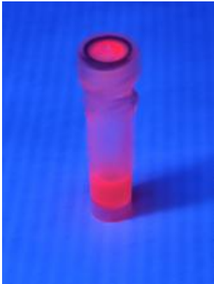
图1 量子点荧光微球在365 nm紫外光激发下发出红光 Fig.1 Quantum dot fluorescent microspheres emit red light under UV excitation at 365 nm
