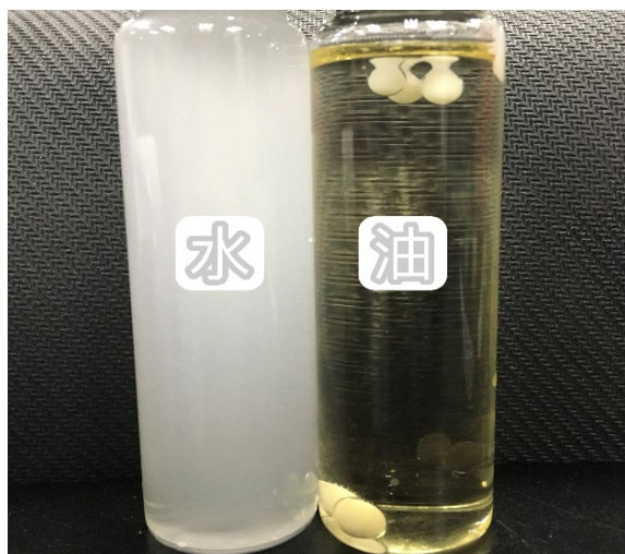
图 1 皮克林乳液类型判断 Fig.1 Type of Pickering emulsion
