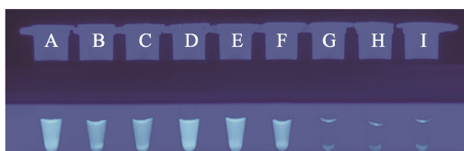
Fig.6 Experimental results on that sensitivity of Vibrio vulnificus detection by LAMP fluorometry
