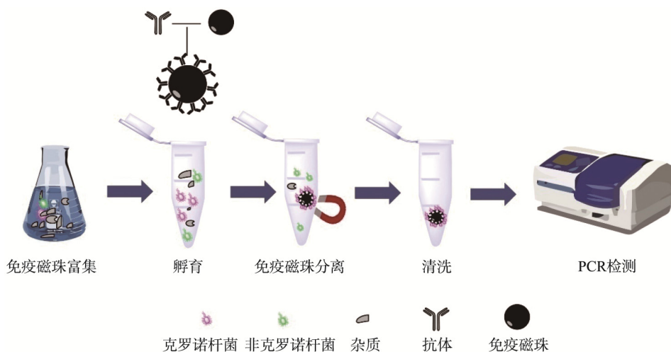
图 3 免疫磁珠富集菌体过程 Fig.3 Enrichment of Cronobacter spp. by immunomagnetic beads
