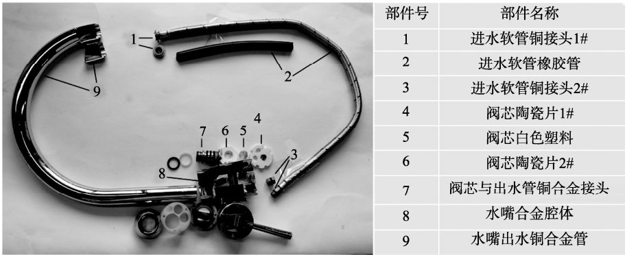
图 2 陶瓷片密封水嘴部件 Fig.2 Parts of the ceramic cartridge faucets
