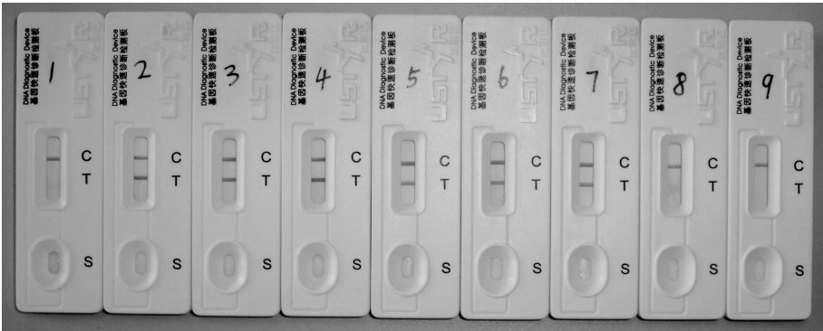
注:1:空白对照;2: 7.1 \times 10^7 cfu/ml;3: 7.1 \times 10^6 cfu/ml;4: 7.1 \times 10^5 cfu/ml;5: 7.1 \times 10^4 cfu/ml; 6: 7.1 \times 10^3 cfu/ml;7: 7.1 \times 10^2 cfu/ml;8: 7.1 \times 10^1 cfu/ml;9: 7.1 \times 10^0 cfu/ml。
